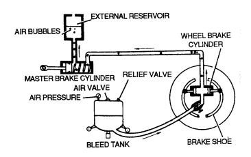
Figure 9-12. Pressure Method of Bleeding Brakes
