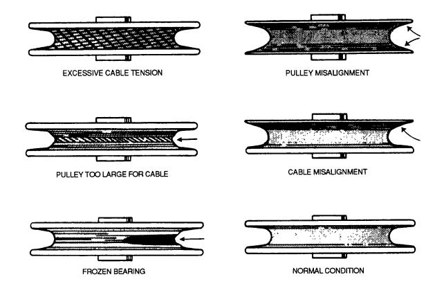
Figure 9-28. Pulley Wear Patterns
