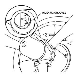
Figure 7-17. Built-In Timing Marks
