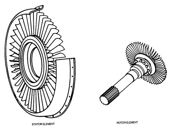
Figure 8-10. Turbine Assembly Elements
