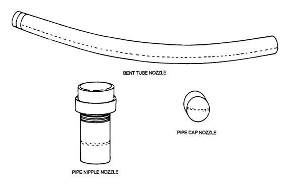
Figure 10-1. Types of Spray Nozzles
