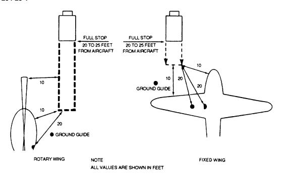
Figure 3-5. Fuel Truck Backing Approach
