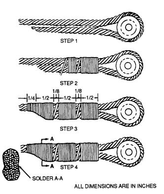
Figure 9-24. Wrapped Solder Splice
