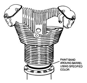
Figure 7-12. Marking of Cylinder
