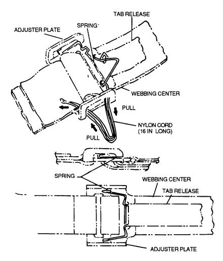
Figure 11-7. Shoulder Harness Webbing Retarder Spring Installation
