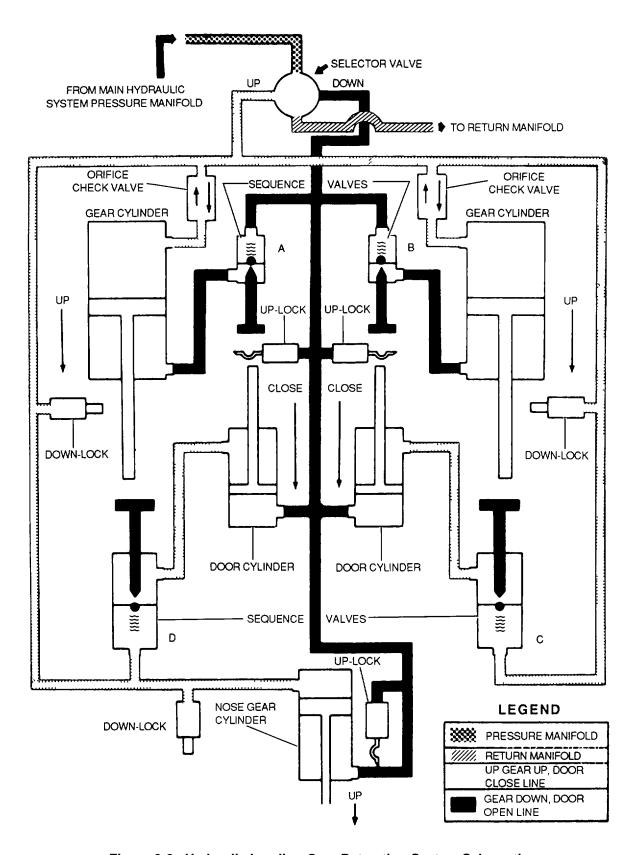
Figure 9-2. Hydraulic Landing Gear Retraction System Schematic
