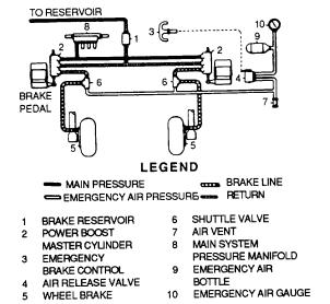
Figure 9-9. Power Boost Brake System
