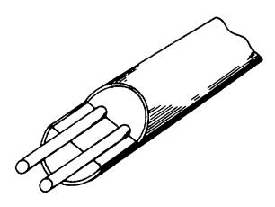
Figure 9-33. Kidde Sensing Element
