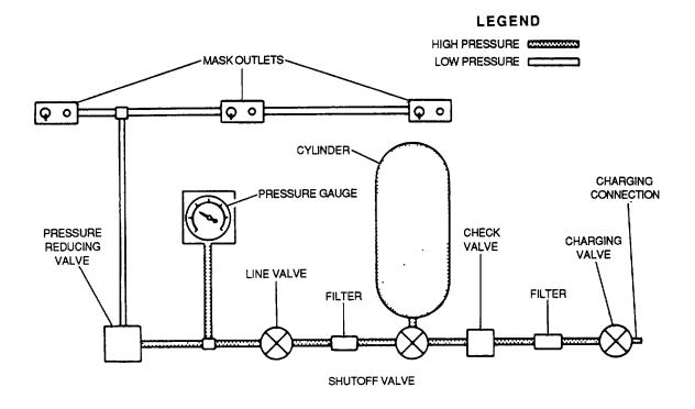
Figure 9-35. Continuous Flow Oxygen System
