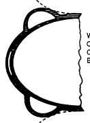
WHEN CENTER CELL DEFLATES, OUTER CELLS INFLATE THIS RAISES CRACKED ICE CAUSING IT TO BE BLOWN OFF BY AIR STREAM
