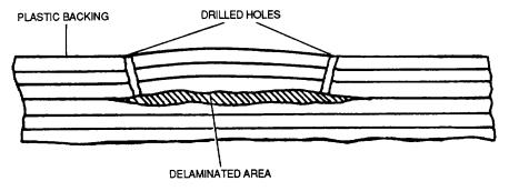
Figure 9-38. Delaminated Repair
