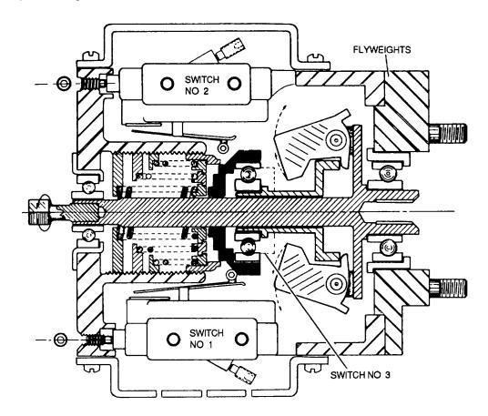
Figure 8-11. Speed-Sensitive Control
