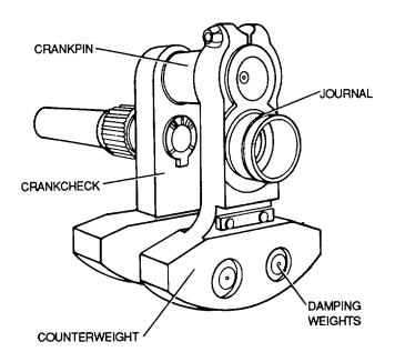
Figure 7-7. Radial-Type Crankshaft (Single-Throw)
