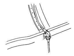
Figure 8-19. Turbine Discharge Pressure Pickup Line
