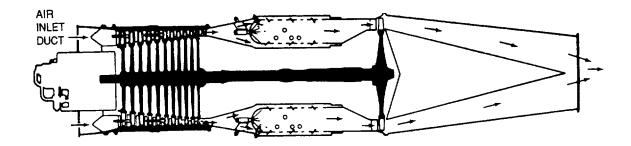
Figure 8-3. Single Entrance Inlet Duct (Axial-Flow Engine)
