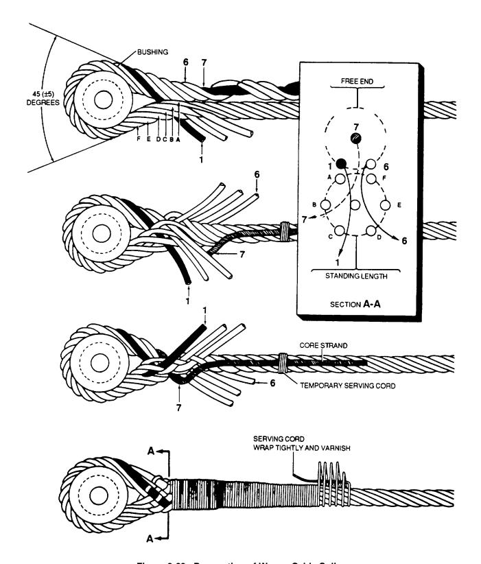
Figure 9-23. Preparation of Woven Cable Splice
