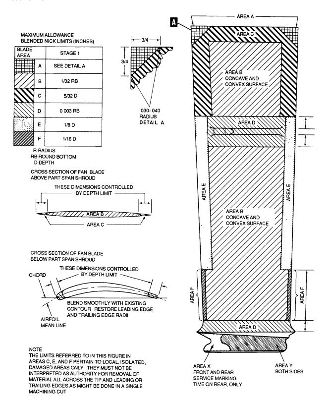
Figure 8-18. Typical Compressor Blade Repair Limits
