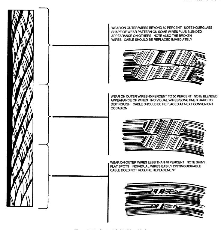
Figure 9-21. Control Cable Wear Limits
