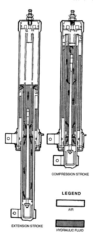
Figure 9-6. Shock Strut Operation
