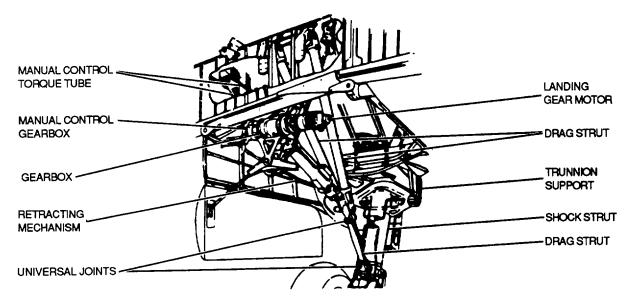
Figure 9-1. Electric Retraction System
