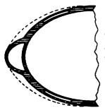
AFTER DEICER SYSTEM HAS BEEN PUT INTO OPERATION, CENTER CELL INFLATES, CRACKING ICE
