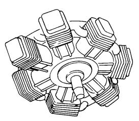
Figure 7-1. Radial-Type Engine
