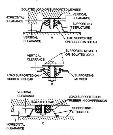
Figure 9-40. Open-Type Vibration Isolators
