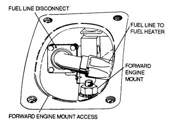
Figure 8-21. Fuel Line Disconnect
