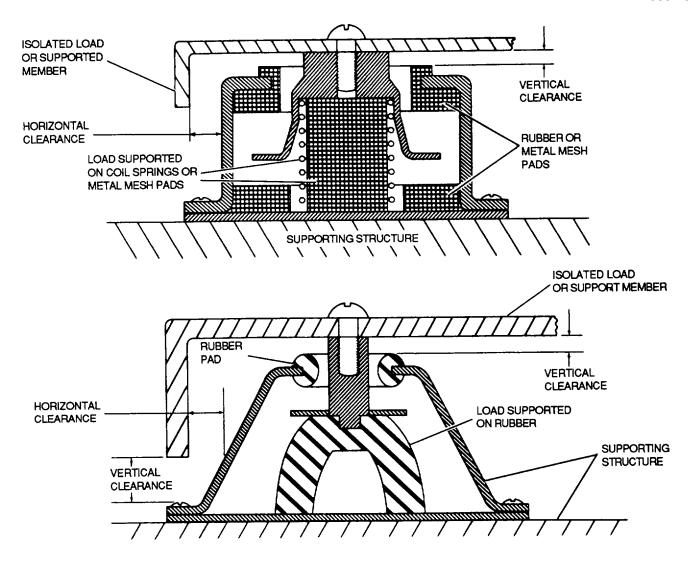
Figure 9-41. Closed-Type Vibration Isolators
