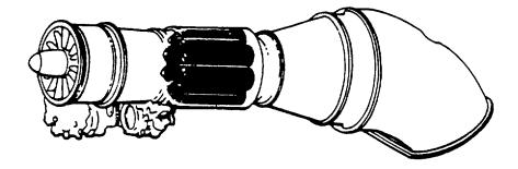
Figure 8-8. Can-Type Combustion Chamber Arrangement
