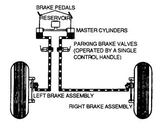
Figure 9-7. Independent Brake System
