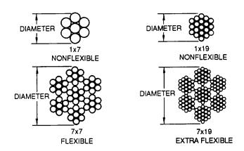
Figure 9-18. Cable Cross Sections
