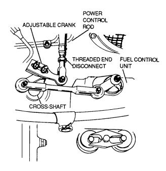
Figure 8-22. Power Lever Disconnect
