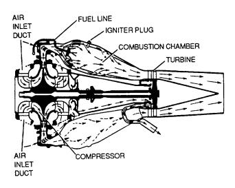
Figure 8-4. Divided Entrance Inlet Duct (Centrifugal-Flow Engine)
