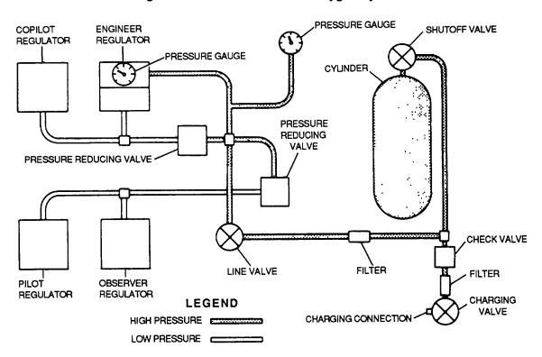
Figure 9-36. Pressure-Demand Oxygen System
