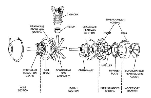
Figure 7-5. Radial-Type Crankcase
