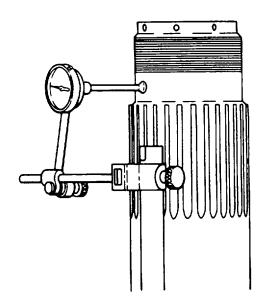
Figure 7-21. Checking Propeller Shaft Runout
