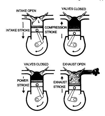
Figure 7-3. Reciprocating Engine Operating Cycle (Four-Stroke)
