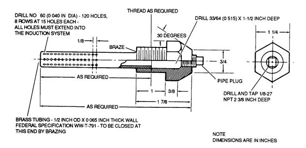
Figure 7-24. Discharge Nozzle for Corrosion Preventive Mixture
