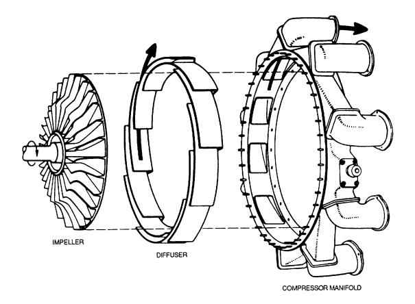
Figure 8-6. Centrifugal-Flow Compressor Components
