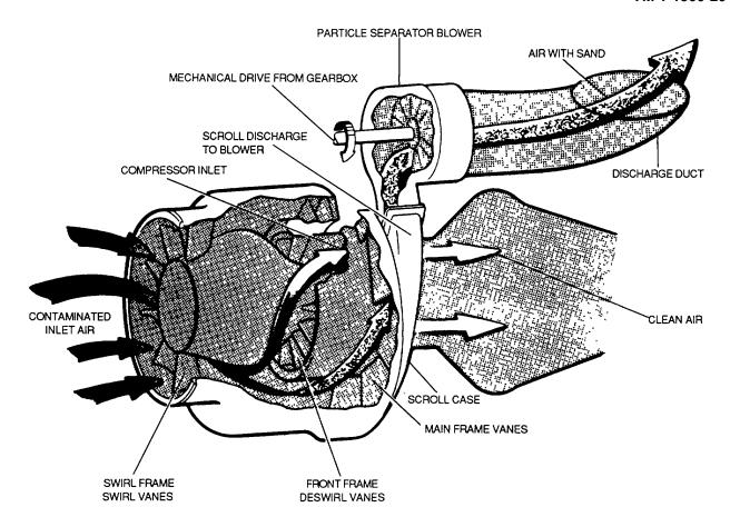
Figure 8-5. Particle Separator
