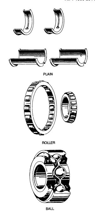
Figure 7-8. Bearing Types
