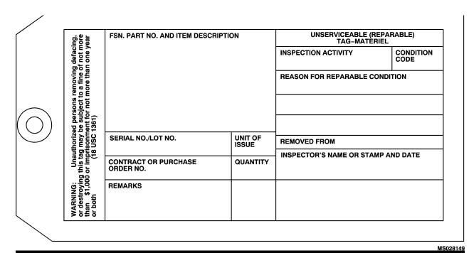
Figure 11-4. Unserviceable (Repairable) Tag-Material (DD Form 1577-2) (Green).
