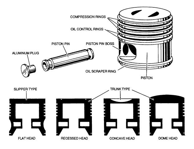
Figure 7-10. Piston, Pin, and Ring Assemblies
