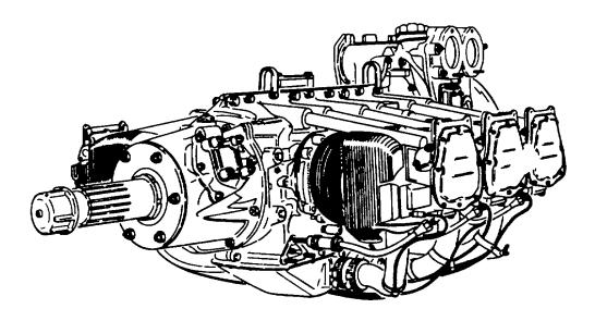
Figure 7-2. Opposed-Type Engine
