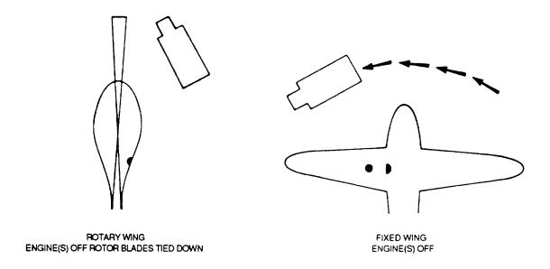
Figure 3-4. Fuel Truck Required Spacing
