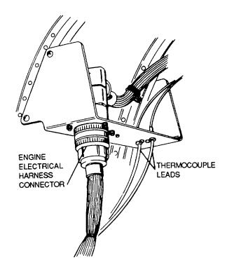
Figure 8-20. Electrical Disconnect
