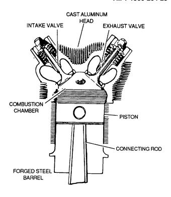
Figure 7-11. Cylinder Assembly
