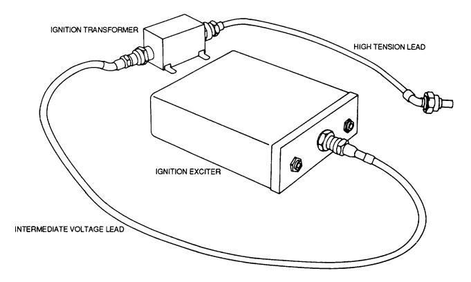
Figure 8-13. One Side of a Typical Ignition System
