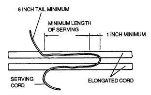
Figure 9-44. Preparation for Serving Shock Cord
