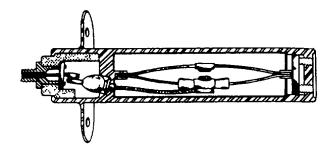
Figure 9-32. Thermal Switch
