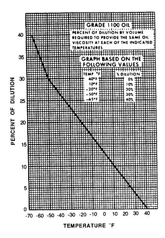
Figure 7-25. Percent Dilution Versus Temperature for Grade 1100 Oil
