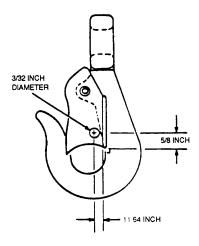
Figure 11-9. Snap Hook Safety Guard Drill Details
