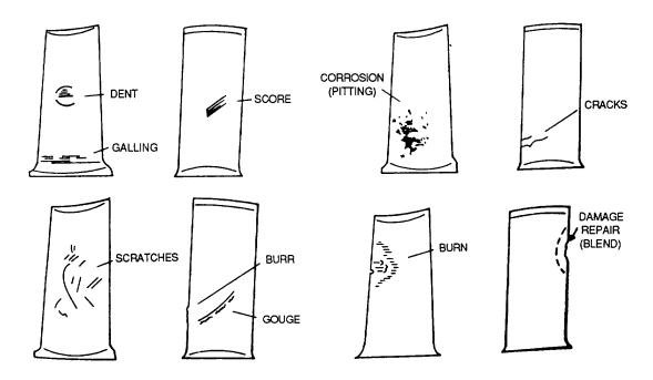
Figure 8-17. Compressor Blade Damage
