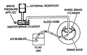
Figure 9-11. Gravity Method of Bleeding Brakes
