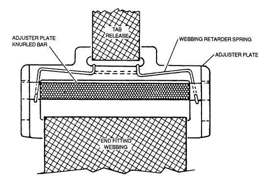
Figure 11-8. Seat belt webbing retarder spring installation
