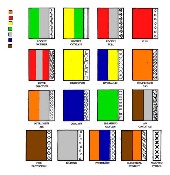
THE ABOVE COLOR CODES REPRESENT DESIGNATION FOR SYSTEMS ONLY FOR CODING LINES WHICH DO NOT FALL INTO ONE OF THESE SYSTEMS, THE CONTENTS SHALL BE DESIGNATED BY BLACK LETTERING ON A WHITE TAPE.
