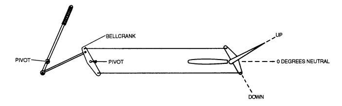
Figure 9-14. Elevator Action
