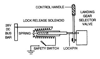
Figure 9-3. Landing Gear Safety Circuit
