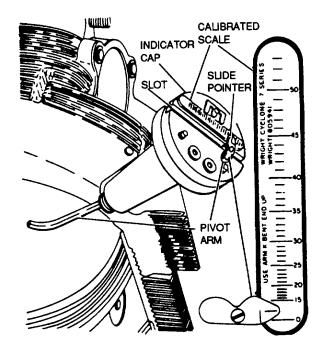
Figure 7-16. Installation of Piston Position Indicators
