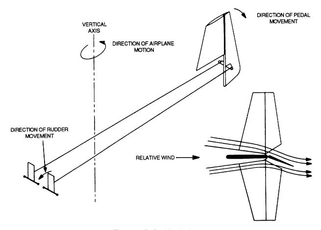
Figure 9-15. Rudder Actlon
