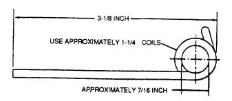
Figure 11-10. Snap Hook Safety Pin Construction
