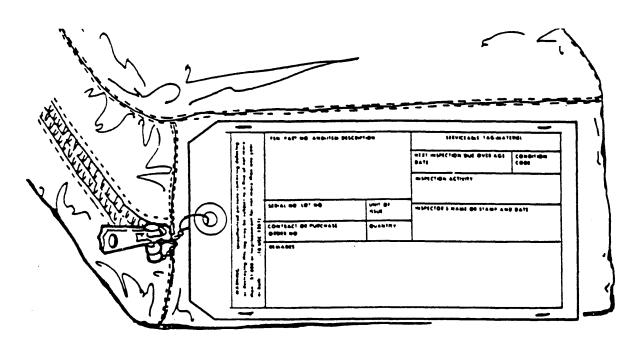
Figure 11-5. Properly Attached Flat-Head Pin, Lead Seal, and Identification Tag.
