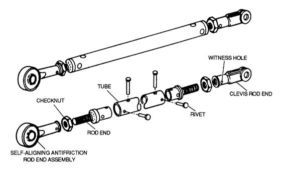
Figure 9-29. Control Tube Assembly
