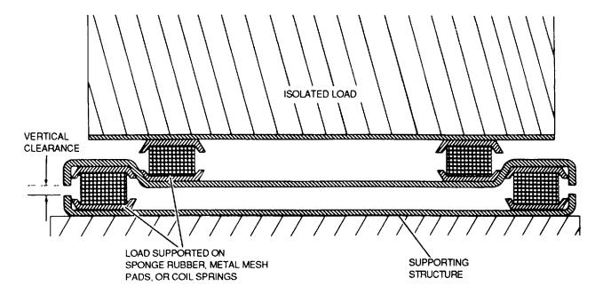
Figure 9-42. Combined Vibration Isolator Mounting Base
