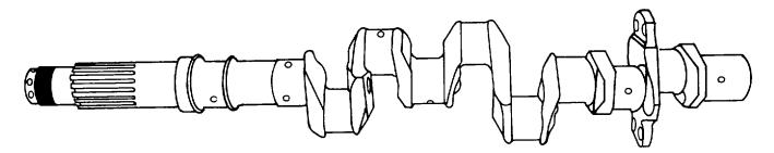
Figure 7-6. Opposed-Type Crankshaft (Six-Cylinder) (Six-Throw)
