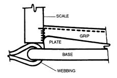
Figure 11-6. Measuring Fingertip Clearance
